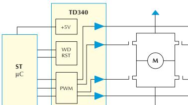
**TD340** Thanks to its 5V regulator and watchdog/reset circuits, the TD340 enables you to build a complete DC motor control system with only a few parts.
