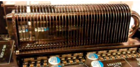
Example: Motherboard (PCB 4 layer, 35 \mu\text{m} ) with high performance heatsink
