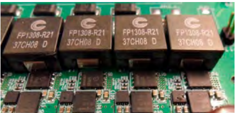
Example: High performance Server (PCB: 8 layer, 70 \mu\text{m} )
