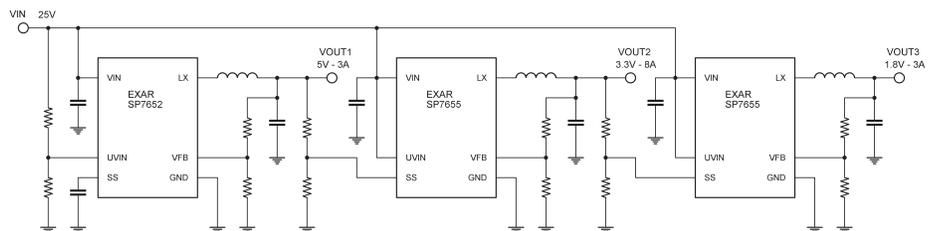
All converters begin their soft start cycle simultaneously with the same slew rate
