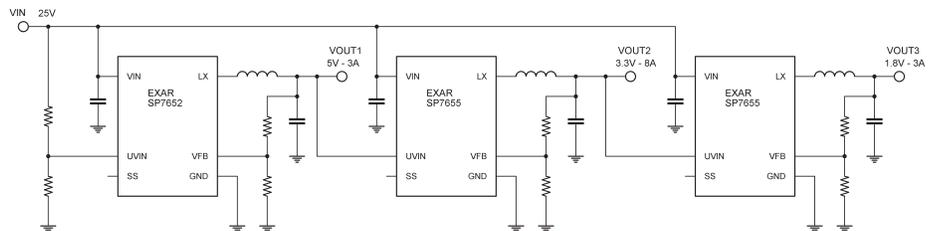
Vout1 powers up first then triggers Vout2 which powers up and triggers Vout3
