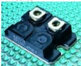
100 and 250 watts. Thick film power resistors designed for heatsink mounting. Very low inductance for high frequency applications. M4 mechanical connections. Request datasheet 100watt 500 250 watt 615
