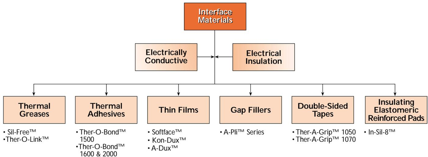
**A-Dux**, when you need thermal conductivity but electrical isolation is important too, A-Dux fits the bill. With the performance of a grease, A-Dux has a breakdown voltage of 250 volts/mil of thickness. This material significantly enhances thermal conductivity between semiconductor packages and heat sinks, and withstands aqueous washing that may occur during the manufacturing process. For faster manufacturing time, have Aavid pre-install A-Dux on your heat sink.
